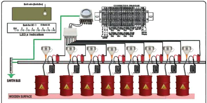
Earth Relay Unit should be connected through Dedicated Earth Pit (Customer Scope)
